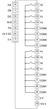
In order to improve EMC performance, bond the FG terminal to ground. Caution: FG terminal is NOT a protective conductor terminal.
