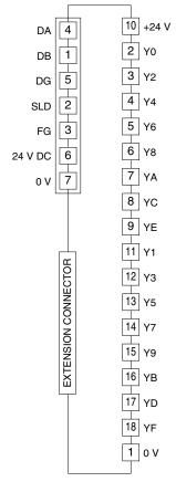
In order to improve EMC performance, bond the FG terminal to ground. Caution: FG terminal is NOT a protective conductor terminal.
