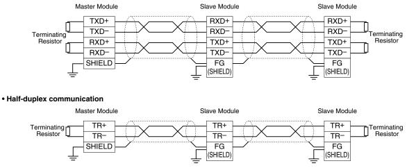
Note: Be sure to turn ON the switch of the terminating resistor located at both ends of the modules.
