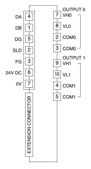
In order to improve EMC performance, bond the FG terminal to ground. Caution: FG terminal is NOT a protective conductor terminal.
