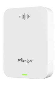
GS301 is a 4-in-1 LoRaWAN® bathroom odor detector to detect ammonia (NH<sub>3</sub>) and hydrogen sulfide (H<sub>2</sub>S) gas according to electrochemical principle. GS301 is also able to detect temperature and humidity to fully aware of the environment of bathrooms. When the NH3 or H<sub>2</sub>S gas concentration reaches the preset threshold, the detector will trigger both LED light alarm and buzzer to notify people timely to ventilate, which is an important part in smart bathroom solution.
